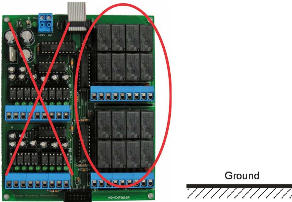
Figure 3 - Incorrect EXP1616R Orientation
