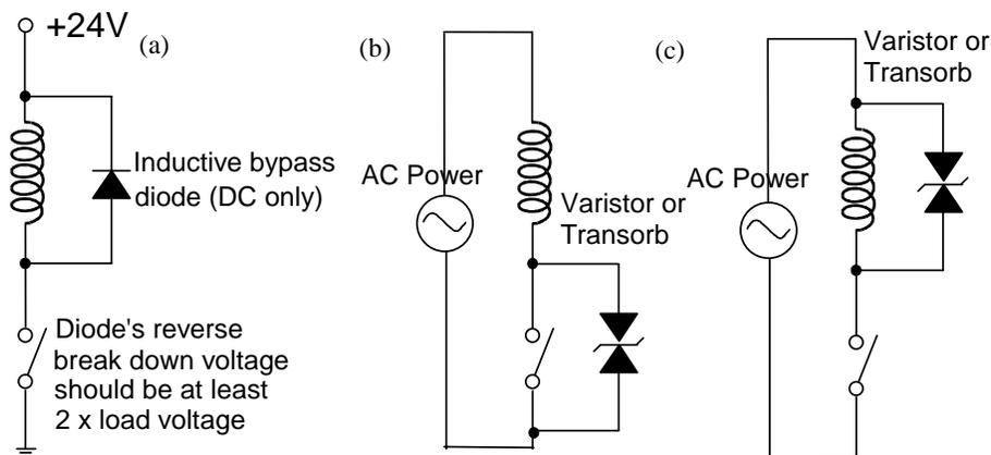
Figure 7 - (a) Inductive snubber circuit - DC load only.
