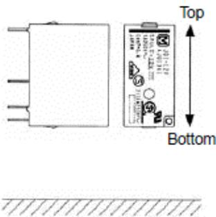
Figure 2 - Incorrect Relay Position
