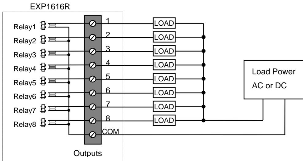
Figure 6 - Relay Output interfacing to load
