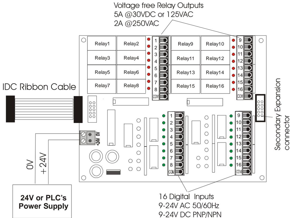
Figure 1 - 32 I/O Expansion board for FMD and F-Series PLCs
